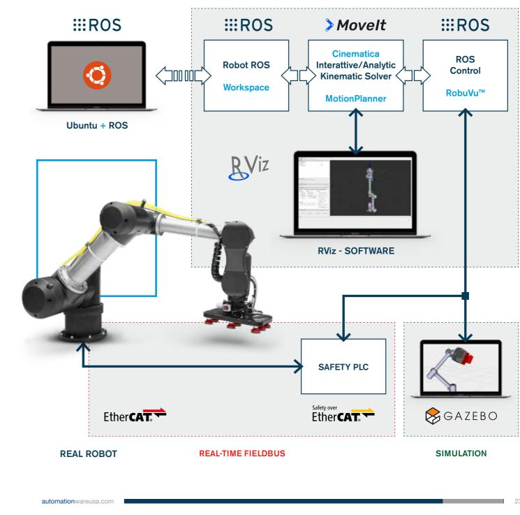
AutomationWare developed a software architecture based on ROS2 to manage their robotic arms (AWTube) and robotic joints (J-Actuator).
